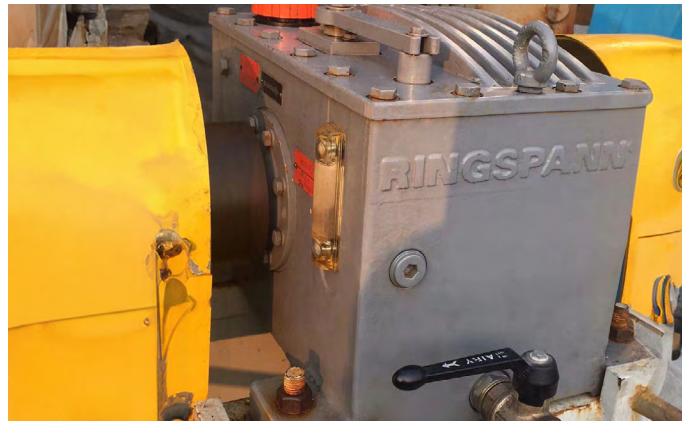
Housing Freewheel FH 1000 in hydraulic turbine pump
