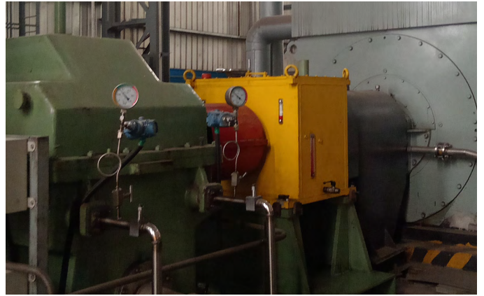
Housing Freewheel FH 60000 in fan drive
