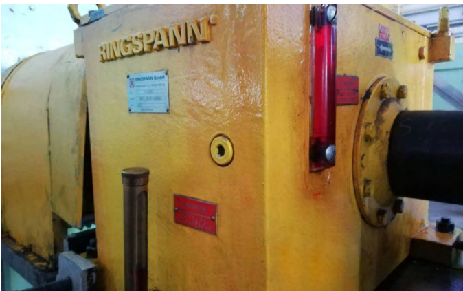
Housing Freewheel FH 4000 in hydraulic turbine pump
